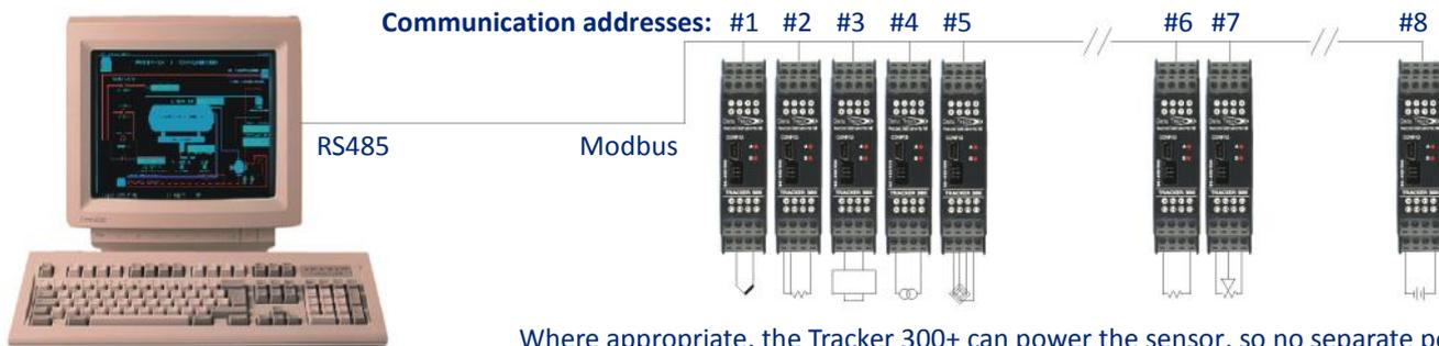
Where appropriate, the Tracker 300+ can power the sensor, so no separate power supply unit is required. Loop power (24VDC) and bridge excitation (10VDC) is provided as standard on the Tracker 321 data acquisition module and the Tracker 332 PID controller.
